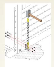
To minimise the risk of wind damage, all arks need to be secured to the ground. We recommend our ground anchor kits are used in all installations bar those on very sandy soils and concrete. It is the customers responsibility to ensure the building is adequately secured.
